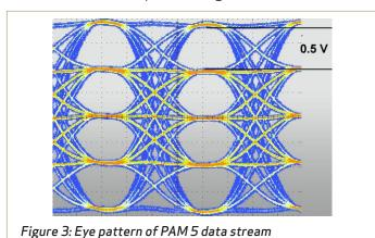
becomes very important. The PAM 5 encoding scheme allows efficient use of bandwidth, but the sacrifice is in SNR sensitivity. So the specifications for 1000BaseT are much more concerned with noise generation than those for 100BaseTx (Fast Ethernet).
