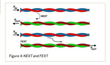
Noise produced by other adjacent "alien" cables is also important. Information about this noise is not available to the noise canceler so it is important to reduce the alien noise to the specification level as defined in Clause 40.7.6: "Measured at the output of a filter connected to the output of the near end of a disturbed duplex channel the noise should not exceed 40 mV peak-to-peak. The filter for this measurement is a fifth order Butterworth filter with a 3 dB cutoff at 100 MHz."
