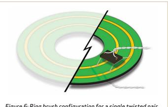
Figure 6: Ring brush configuration for a single twisted pair
