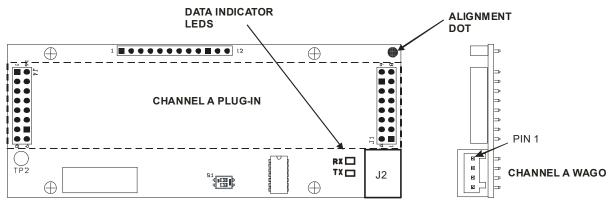
Figure 2-6: 914-AIB Adapter Card
