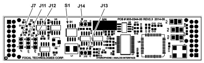
Figure 4-5: AIB Hydrophone Plug-In Module
