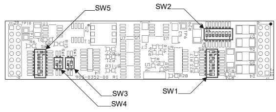
Figure 4-2: AIB RS-485 Plug-In Module
