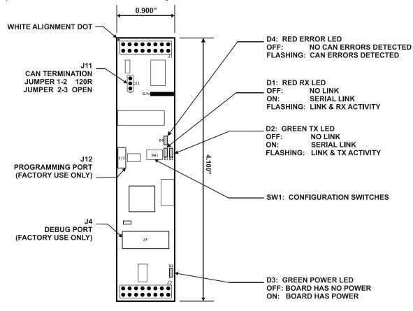
Figure 4-7: AIB-CANBUS Plug-In Module (Top View)
