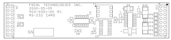
Figure 4-1: AIB RS-232 Plug-In Module
