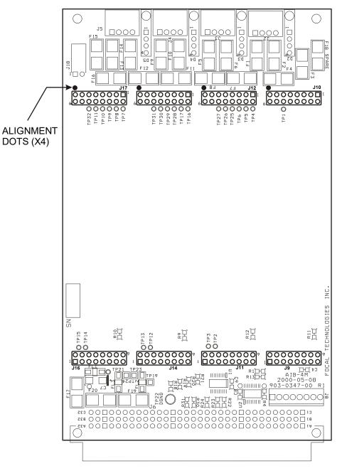
Figure 2-2: Model 903 AIB-4 Motherboard (AIB-4M)
