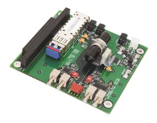
The 907-ECL (Emitter Coupled Logic) media converter provides optical transmission of high speed data formats typically used by sonars over a singlemode or multimode fiber. This card may be switch configured to support single-ended and differential ECL/PECL signals.
