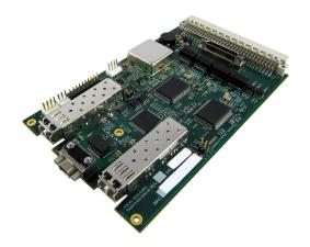
The Model 922-FOM is a lightly managed Ethernet switch designed and tested for use in subsea controls and communication applications. With five copper Ethernet ports and two optical Ethernet ports, the FOM may be operated with both optical ports and (optionally) one copper port configured for redundant operation, so that the failure of one link automatically and rapidly redirects traffic to one of the other ports in a protocol independent manner.
