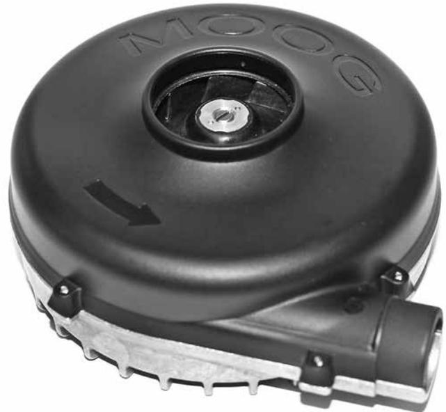
The Moog AirMax™ P28 series of fans and blowers provides excellent output power per unit volume through the use of compact, high energy 3-phase brushless DC motors and efficient airfoil design. The motor utilizes high energy rare earth magnets to provide the blower with the necessary torque to provide maximum airflow in the minimum amount of system space.
