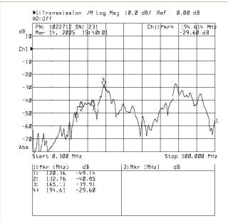
Figure 10: Crosstalk vs frequency in slip ring assemblies
