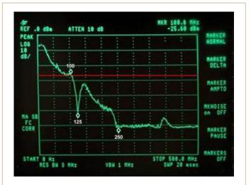
Figure 4: Frequency spectrum of 100BaseT-Ethernet
