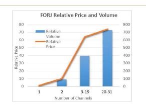
Figure 18: This figure shows the relative difference in price and volume of multi-channel FORJs compared to a single channel FORJ (relative values of 1). These differences occur in jumps.
