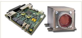
Figure 20: Two examples of multiplexers are shown. A board level multiplexer that supports multiple uncompressed HD video channels, multiple serial data channels and a single Gigabit Ethernet port. A small Camera Link® multiplexer is shown that converts copper Camera Link signals into a single fiber channel.
