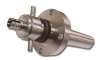
The FO197S is a sealed single-channel multimode fiber optic rotary joint (FORJ) which is passive and bidirectional, and allows the transfer of analog or digital optical signals across rotational interfaces. The FO197S is specially designed for durable, corrosion free use when exposed to harsh outdoor environments.
