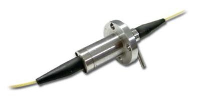
The FO285 (single-channel singlemode) and the FO286 (single-channel multimode) are passive and bidirectional, and allow the transfer of optical signals across rotational interfaces. Both models also offer other benefits of fiber optics, including low spark hazard.
