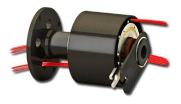
The Model 813 electrical and fluid rotary union consists of a single fluid pass with 600 V / 10 A and 220 V / 2 A power / signal circuit combinations. The design features sealed-for-life rolling element bearings and fiber brush technology for ultimate performance and long, maintenance free life in many challenging applications.
