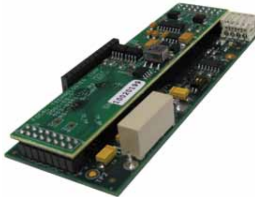
914-AIB Adaptor Board Supports Any AIB Daughter-card Plug-in
