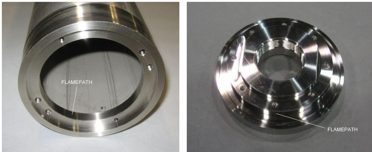
Figure 10b – Flamepath surfaces. It is critical that these surfaces not be damaged during removal and replacement of the COVER ASSEMBLY.
