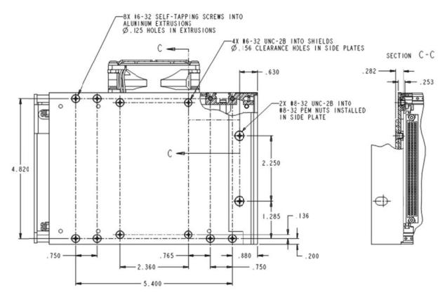
Figure 8.1-1: Side View of Typical Model 903 Console Card Cage
