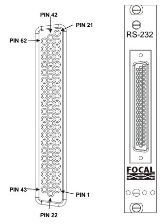
Figure 5.2-1: DIB-232-16 High Density RS-232 Board
