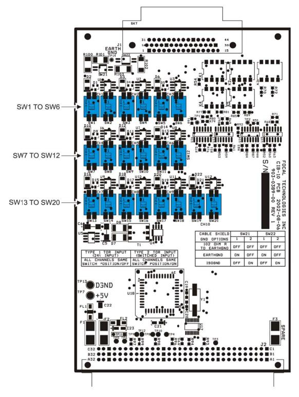
Figure 5.4-3 shows a view of the CIB-10 PCBA with location of configuration switches.
