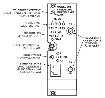
Figure 3.1-3: Console FMB-X-2.5 Front Panel
