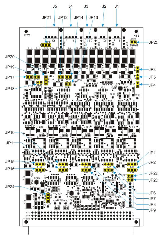
JP22 and JP23 should remain shunted at all times. JP24 should have pins 1-2 shunted at all times. JP25 is a spare shunt.
