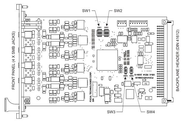
Figure 4.1-3: VIB-X Plan View
