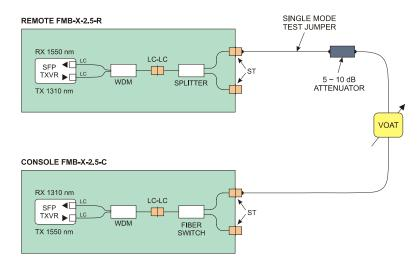
Figure 8.4-2: Flux Budget Test Setup – Link Threshold Measurement
