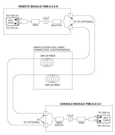
Figure 2.3-1: Model 903 Fiber Optic Transmission System
