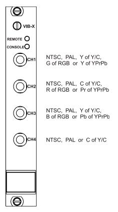
Figure 4.1-2: VIB-X Front Panel
