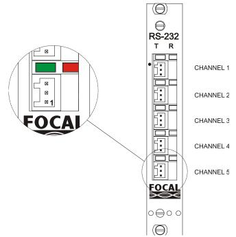
Figure 5.1-1: DIB-232 Front Panel
