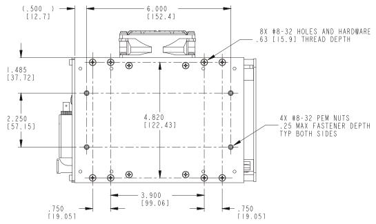
Figure 8.1-2: Side View of Typical Model 903 Remote Card Cage
