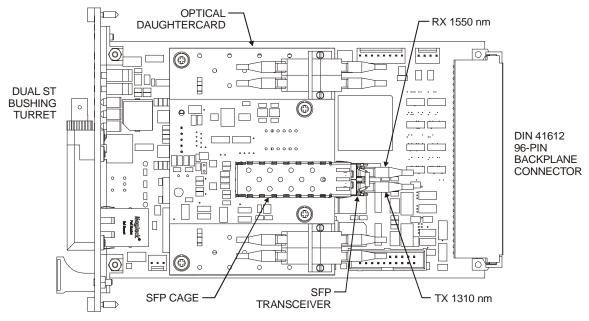
Figure 3.1-2: Remote FMB-X-2.5 Plan View
