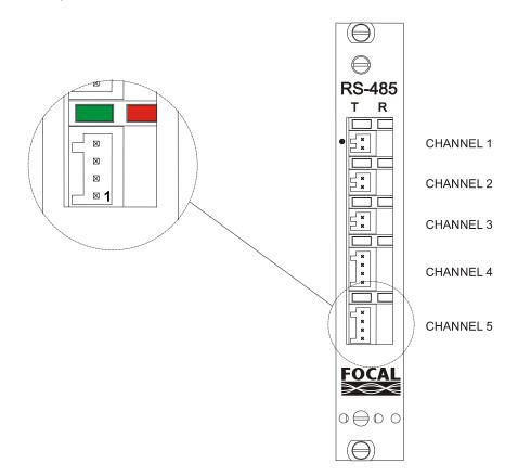
Figure 5.3-1: DIB-485 Front Panel
