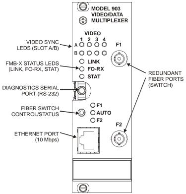
Figure D.2-1: Console GLINK FMB-X Front Panel
