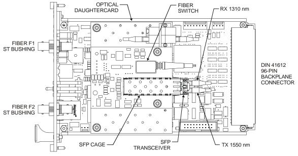
Figure 3.1-4: Console FMB-X-2.5 Plan View
