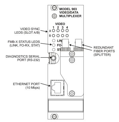
Figure D.1-1: Remote GLINK FMB-X Front Panel View
