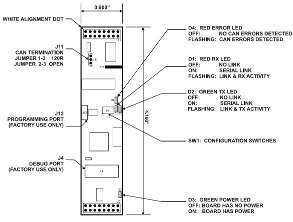
Figure 5.6-10: AIB-CANBUS Plug-In Module (Top View)
