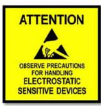
Grounded ESD wrist straps must be worn and proper ESD safety precautions observed when handling printed circuit boards.
