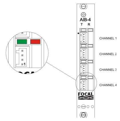
Figure 5.6-1: Adaptable Interface Board (AIB-4) Front Panel
