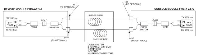
Figure 7.2-1: Block Diagram of Model 903 Fiber Optic Transmission System
