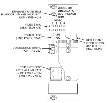
Figure 3.1-1: Remote FMB-X-2.5 Front Panel View
