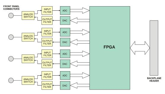
Figure 4.1-1: Block Diagram of VIB-X Card
