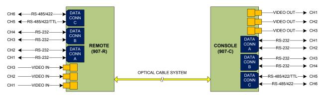
Figure 3-3: On board I/O Channels for 907-R and 907-C Multiplexer Motherboard Cards
