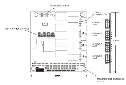
Figure 5-4: 907-SER, Serial Data Expansion Card
