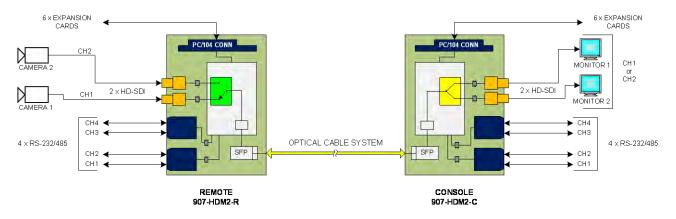
Figure 3-15: On board I/O Channels for 907-HDM2-R and 907-HDM2-C Multiplexer Motherboard Cards (Single Video Channel – Full Sampling, Switched Dual Input)
