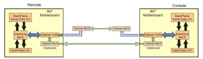
Figure 3-1: Remote & Console Motherboard Optical Configuration
