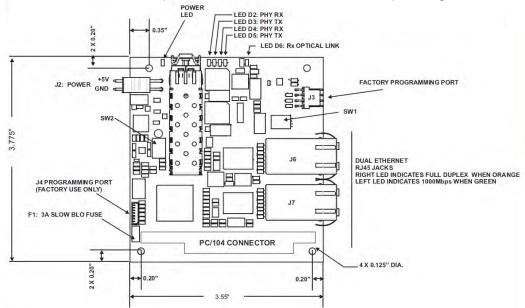
Figure 4-7: 907-GBE2, Dual Gigabit Ethernet Media Converter Card
