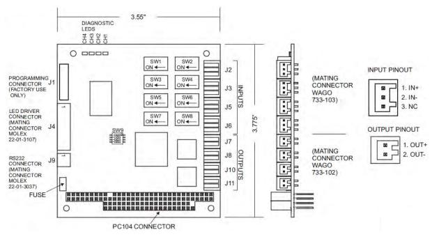
Figure 5-10: 907-CIB Control Channel Expansion Card
