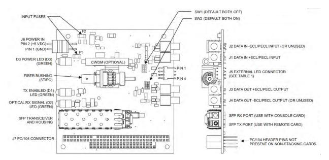
The 907-ECL cards are available in pressure tolerant versions with a 6000 psi rating.
