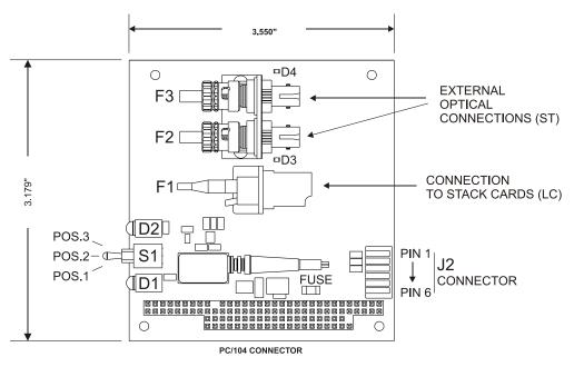
Figure 6-8: 907-FOS, 1x2 Fiber Optic Switch Card
