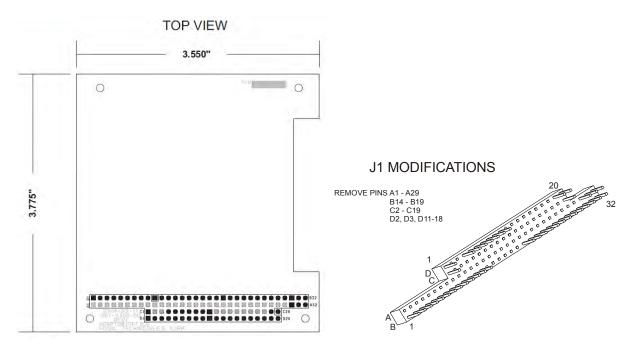
Figure 6-3: 907-PC104, 907 to Standard PC/104 Adaptor
