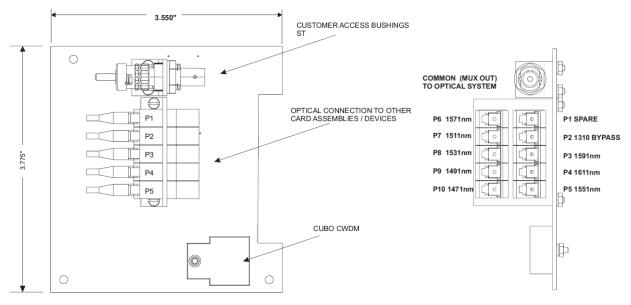
Figure 6-7: 907-CWDM-8, 8-Channel CWDM Optics Card
