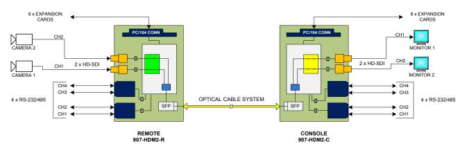
Figure 3-13: On board I/O Channels for 907-HDM2-R and 907-HDM2-C Multiplexer Motherboard Cards (Dual Video Channel – Optimized Sampling) Option B: 907-HDM2 Dual Video (Full Sampling), factory modification option.
