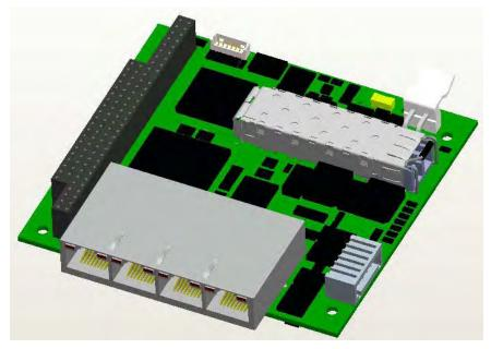
Figure 4-1 shows a Quad-port Gigabit Ethernet Switch (GBES) media converter card.
