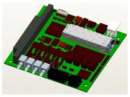
Figure 3-8: Model 907Plus Multiplexer Motherboard
