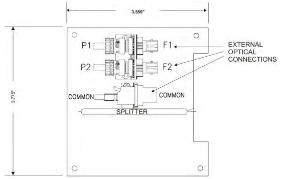
Figure 6-9: 907-SPLIT, 1x2 Optical Splitter Card
