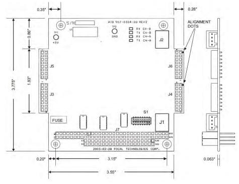
Figure 5-13: 907-AIB, Adaptable Interface Board Adaptor
