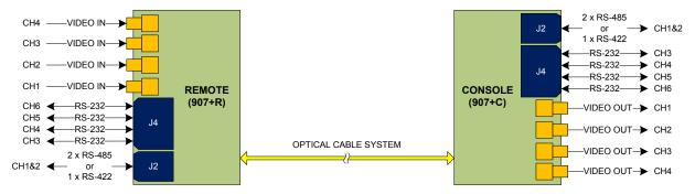
Figure 3-9: On board I/O Channels for 907+R and 907+C Multiplexer Motherboard Cards
