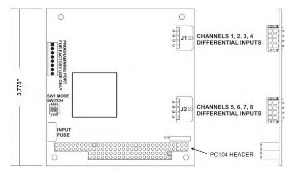
Figure 5-5: 907-ADC Expansion Card
