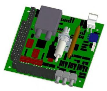
Figure 3-2: Standard Model 907 Multiplexer Motherboard with WDM
