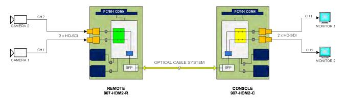
Figure 3-14: On board I/O Channels for 907-HDM2-R and 907-HDM2-C Multiplexer Motherboard Cards (Dual Video Channel – Full Sampling)
