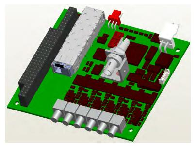
Figure 3-5: Model 907V Multiplexer Motherboard
