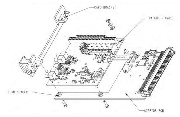
The 907 Eurocard adaptor PCBA can be configured with either a 4HP- or 8HP-wide front panel for a 3U Eurocard rack. Figure 6-2 shows a 907-EURO Eurocard adaptor card assembly.
