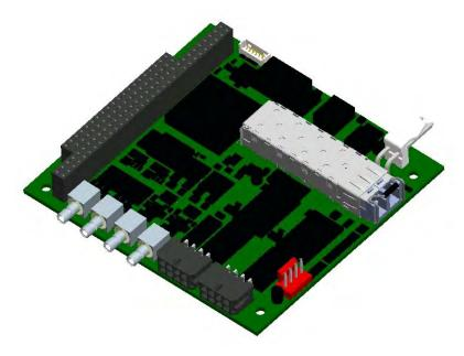
Figure 3-12: Model 907-HDM2 Multiplexer Motherboard
