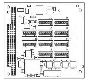
Figure 6-10: 907-DIAG LED Diagnostics Interface Card
