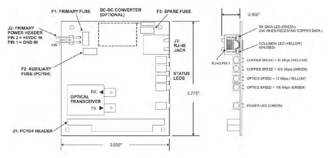
Figure 4-2: 907-MC (10/100 Ethernet) Card without WDM
