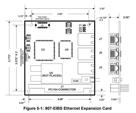
Configure switch SW1 to set the backplane data port used by the 907-EIBS card. All ports (1-6) are available. The default setting is data port #1.
