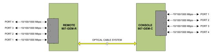
Figure 3-18: On board I/O Channels for 907-GEM-R and 907-GEM-C Multiplexer Motherboard Cards
