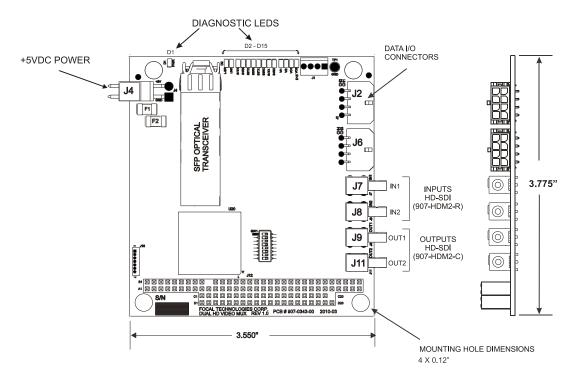
Figure 3-16: 907-HDM2-R & 907-HDM2-C Multiplexer Card
