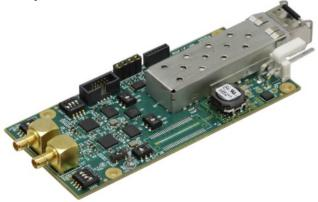
The Moog Focal 914-HDV2 is an extremely compact, ruggedized, single card solution for two high definition (3G/HD-SDI) video channels.
