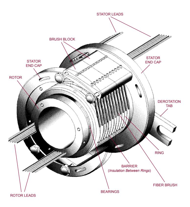
Note: Outer housing is removed for clarity.
