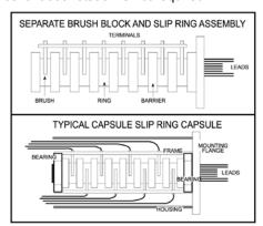
There are two basic slip ring configurations to consider based on space allocation in your system:
