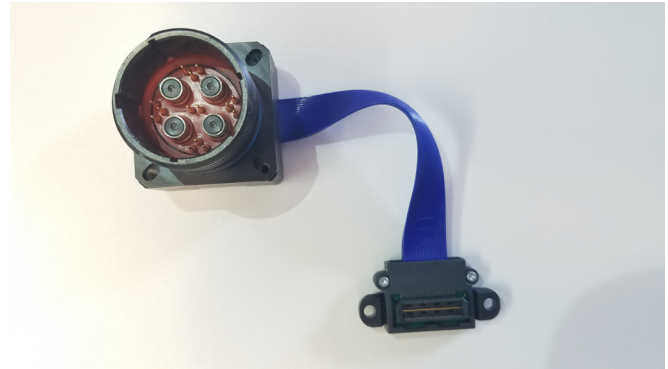
Two duplex optical links operating up to 5Gbps
