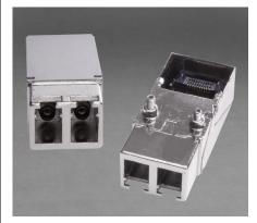
Stiletto series optical fiber transceivers consist of optoelectronic transmitter and receiver functions integrated into a pluggable Duplex LC compliant receptacle connector. The optical transmitters are 850 nM VCSEL lasers. The transmitter input lines are driven with differential CML signals applied to the transmitter (TX+ and TX-) lines. Dual loop, temperature compensated, VCSEL drivers convert the transmitter input signals to suitable VCSEL bias and modulation currents.
