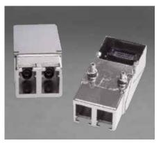
Stiletto series optical fiber transmitters consist of optoelectronic transmitter functions integrated into a pluggable Duplex LC compliant receptacle connector. The optical transmitters are 850 nM VCSEL lasers. The transmitter input lines are driven with differential CML signals applied to the transmitter (TX+ and TX-) lines. Dual loop, temperature compensated, VCSEL drivers convert the transmitter input signals to suitable VCSEL bias and modulation currents.
