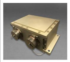
Viking series 8+8 managed Ethernet switches consist of 8x 10/100/1000Base-T ports plus 8x 100Base-FX or 8x 1000Base-SX optical ports in rugged multiport D389999 connectors.
