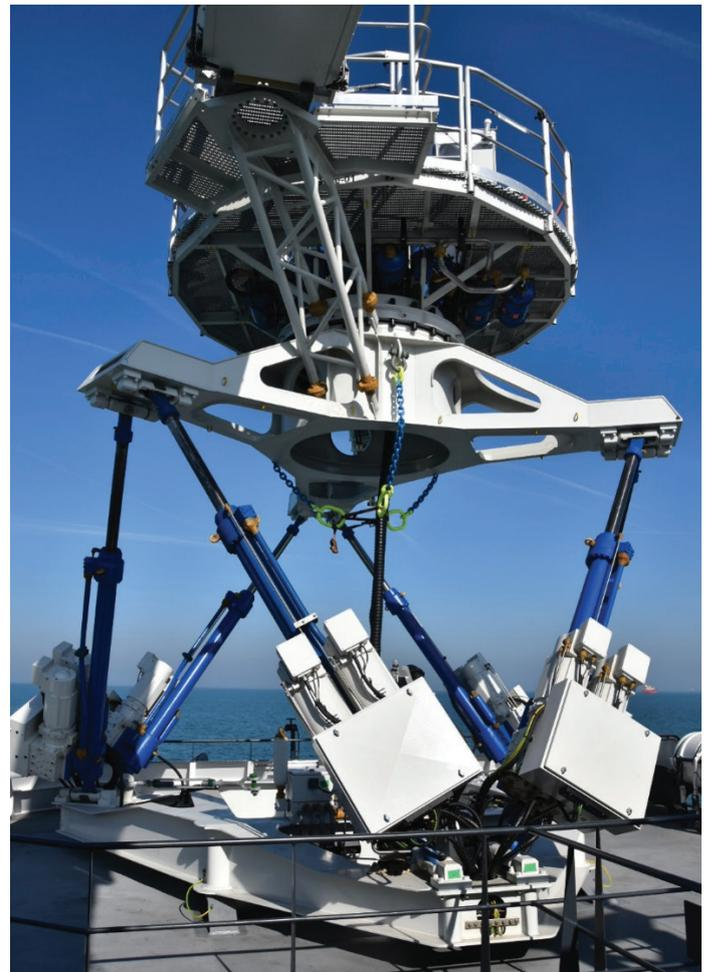
Fig. 1: New Ampelmann A-Type Gangway with EAS
