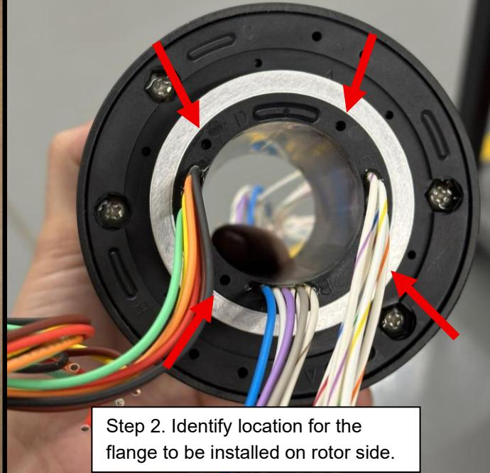
3. Align screw holes of bearing
