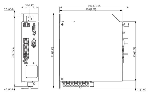
Axis module 75 mm (2.95 in) - Weight 2.3 kg (5.07 lbs)
