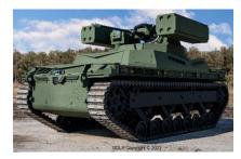
The third RIwP turret on display at AUSA 2023 will be in General Dynamics Land Systems' (GDLS) booth (#6027). This SHORAD RIwP configuration will host a 30mm gun, dual Stinger missile launchers, and a tethered UAS along with radars integrated onto GDLS' Tracked Robot 10-ton (TRX) platform.
