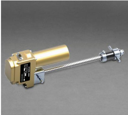
The Model 290 is one of the highest performance linear servo actuators available on the market. We offer this actuator with a digital communications interface. It provides 1,500 lbf at 0.26 inches / second for up to 7.75 inch strokes. It has a homing sequence that determines end of travel on startup, thus, ensuring proper positioning along its stroke. These features allow our customer flexibility to have a drop-in servo actuator for their system.
