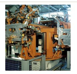
Figure 2: Complex automotive assembly turntable/robot has a fiber optic rotary joint in the center to transfer communication data. EMI isolation of fiber channel is critical in this application. Rotary joint provides power and signal slip rings as well as hydraulic power.
