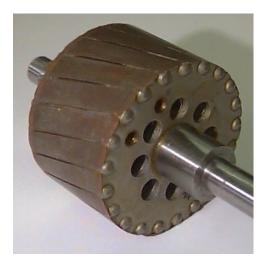
AC Induction motor rotor.
