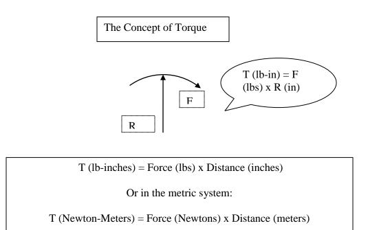
The next important concept in the study of electric motors is the concept of "Power". In a rotating device such as an electric motor, Power has two elements: the rotating force (torque) and the speed at which this power is being applied. The product of torque and speed is the power in watts. This is the same concept electrically, where the power is the product of Volts x Current.
