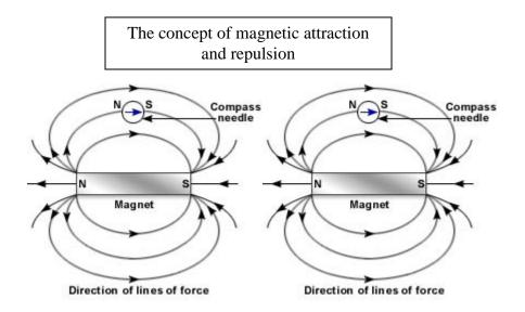
When magnets are brought close to each other, they generate a force of attraction (with adjacent unlike poles) or repulsion (with adjacent like poles). The generation of the mechanical force is fundamental to the way in which all electric motors operate. It can be intuitively seen that to get greater electromagnetic force, the following notions are true:
