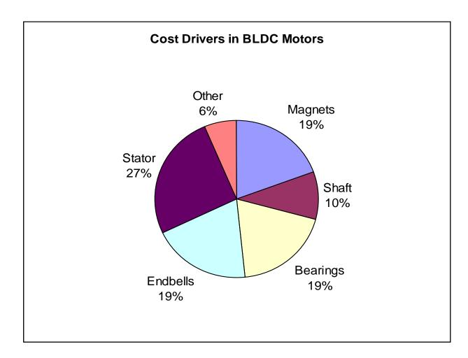
Typically, the cost of the electronics is about as much as the cost of the complete motor. Here again, it may be misleading to generalize but this is a first approximation to give the reader a general idea about the cost and the cost drivers.
