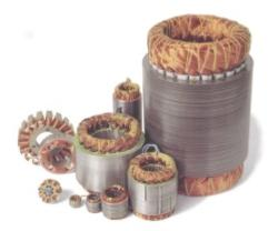
Here are some examples of finished stators, after they are wound. There are optional processes after the winding like varnishing, lacing, shaping the end turns and attaching connectors to the wires, to prepare the wound stacks for final assembly.
