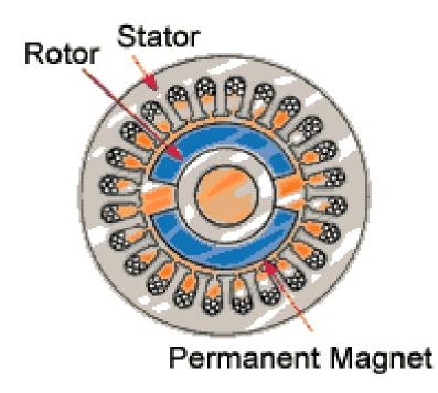
The above is a cross sectional view of a typical brushless DC motor. The permanent magnets are on the inside and on the rotor. The stator is on the outside and has the windings.
