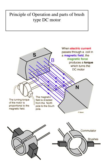
Armature (rotating part or rotor) of a brush type DC motor. The stator is made of a pair or more of permanent magnets or a wound field.
