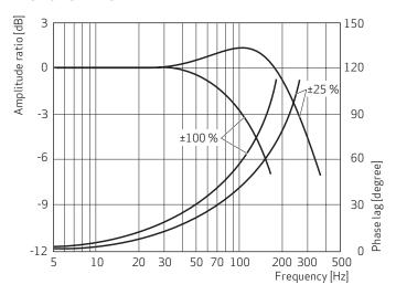
Typical responses for peak sinusoidal inputs of  $\pm 25\,\%$  and  $\pm 100\,\%$  rated current
