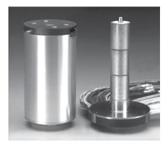
The M series of slip ring assemblies were developed for a wide variety of applications and environments. The M series is an ideal choice for limited space applications. As many as 120 separate circuits are accommodated in a 2.7 inch diameter OD envelope and in less than 5.50 inches long. These slip ring assemblies are a quick turn solution for your application. Off the shelf components allow for a delivery which meets your needs.
