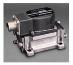
The Type 30 Servo Valves encompass a twostage, flow control, double-nozzle, mechanical feedback design within a rugged stainlesssteel body with an integrated torque motor in an environmentally sealed compartment. Its nozzle-flapper design is a proven technology for military applications where high response, reliability, stability, and accuracy are required within a compact space.
