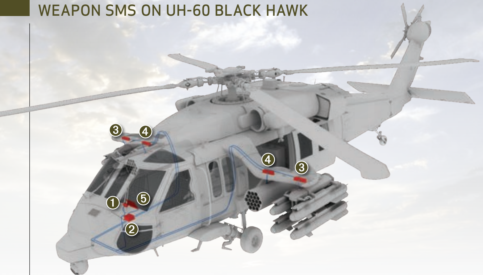
UH-60 Black Hawk Digital SMS Components (Dimensions are in inches)
