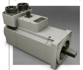
This compact brushless Servo Motor is designed to meet the special requirements of main battle tanks with 2-in-1 stator (double motor) arrangement to accommodate the high power needed. The brushless servo motor is intended to be integrated into a traverse actuator with a gearbox, brake and manual input/ auxiliary drive assembly.
