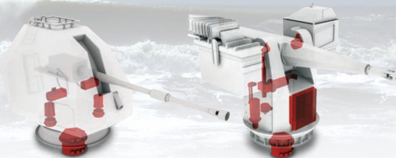
BAE Systems' Mark 8 Mod 1 Naval gun: Moog provides the high performance motors for aiming stabilization and ammunition loading. The slip ring transfers power and data.
