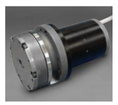
The Moog M8 rotary incremental actuator is a compact, closely integrated design made up of two key elements, a motor and a harmonic drive speed reducer. The motor is a small angle permanent magnet stepper with a relatively high holding torque. The harmonic drive speed reducer offers a large reduction ratio, high load capability, low weight, zero backlash and high torsional stiffness. Coaxial nesting of the
