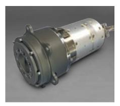
The Moog Type HT-1 Rotary Incremental Actuator is a new addition to the rotary actuator product line. It is a compact, closely integrated coaxial design composed of a small size permanent magnet stepper motor driving the output stage through a gear transmission consisting of a larger size harmonic drive. The actuator provides relatively high holding and running torque for its size. This actuator is optimized for low weight and relatively high
