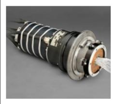
The single axis High Power Solar Array Drive Assembly (SADA) is based on the Type 5 Rotary Incremental Actuator. This standard SADA meets up to 10 kilowatts of power transfer. The design is configured with a Harmonic Drive gear set driven by a Moog discrete permanent magnet stepper motor, potentiometer for position sensing and a high power Twist Capsule assembly for power transfer.
