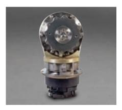
The Type 33 Biaxial Gimbal is of a size appropriate for many antennas, and it has become by far our most popular Antenna Pointing Mechanism configuration. Available in either Elevation/ Azimuth or X/Y, these units have proven their reliability and versatility many times over. Each actuator of the gimbal can incorporate cable management capability. The actuators are based on Moog's heritage Type 3 actuator design with significant on-orbit experience.
