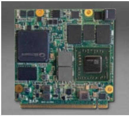
The e2000/e2100 heterogeneous computing product families are radiation tolerant high-performance compute modules for onboard data processing. The products have spaceflight heritage and uses low power embedded x86 compatible AMD® G-series SOC products from the 1st, 2nd, and LX families. The SOC is paired with a powerful Microsemi® SmartFusion2™ FPGA which provides IO expansion and board supervisory management through IP core state-machines or embedded ARM® Cortex™ M3 micro-controller.
