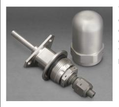
These mechanically operated valves are opened/closed by rotating an actuation nut. The ground connection is a standard AN-style fitting that can be attached prior to operating the valve. The actuation nut, AN cap, and valve cover have tie wire provisions.
