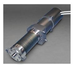
The Cryogenic Fine Positioning Actuator product is designed to produce very small linear output steps using conventional actuator technology. Actuation is accomplished by using a small angle stepper motor coupled to a large gear reduction transmission. The linear excursion is accomplished with a fine/leadscrew mechanism.
