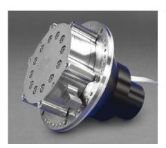
The Moog Micro3 rotary incremental actuator is a compact, closely integrated design made up of two key elements: a rotary actuator and a standard Type 3 speed reducer and output flange. The motor is a small angle permanent magnet stepper with relatively high holding torque. The multistage speed reducer offers a large reduction ratio, low weight, low power consumption,
