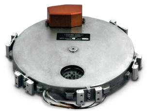
The Cassini Narrow Field FWA housed 24 filters on two disks each having 12 filters with 1.15 inch diameter clear aperture. The Wide Field FWA housed 18 filters on two disks each bearing 9 filters with 1.55 inch diameter clear aperture. Both units are driven by two motors housed in an envelope of 9.00 inches diameter with less than 1.35 inches height.
