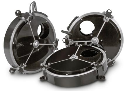
The Fine Guidance Systems FWA is located in the optical path. The FWA assembly consists of a wheel bearing five filters with 2.0 inch diameter clear aperture. These filters are used to minimize the lateral color effects in the FGS astrometer.
