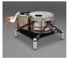
Moog's design of Filter Wheel Assemblies is unique in concept and has been used successfully on several space missions. The design is based on integrating the motor rotor with the optical disk thus providing an optimized solution with high torque in the most compact volume and with lower mass. The more conventional design of filter wheels driven by external motors has the design
