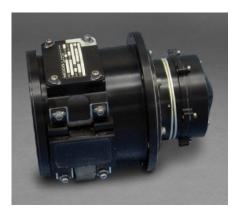
The Type 1 solar array drive assembly offers a minimum weight, minimum power solution for positioning solar array panels at the lower end of the size/power spectrum. It is based on the Moog Type 1 rotary incremental actuator. Continuous rotation of the solar array is facilitated by the integration of a slip ring assembly on the output of the actuator, and the rear accessory section of the Type 1
