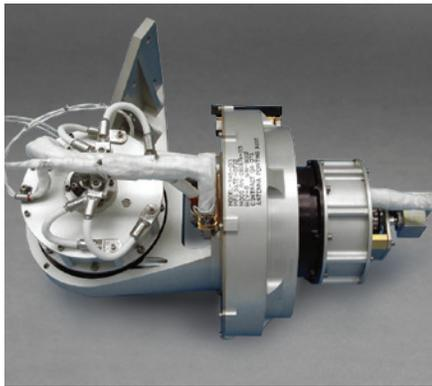
The Type 22 antenna positioner assembly is a compact two-axis gimbal which is ideally suited for supporting and positioning small to medium sized spacecraft communications antennas. It is based on the Moog Type 2 rotary incremental actuator. The gimbal can be configured with either azimuth-elevation or X-Y (crossed axis) geometry, and several approaches to electrical cable management are available. Electrical cables can be carried
