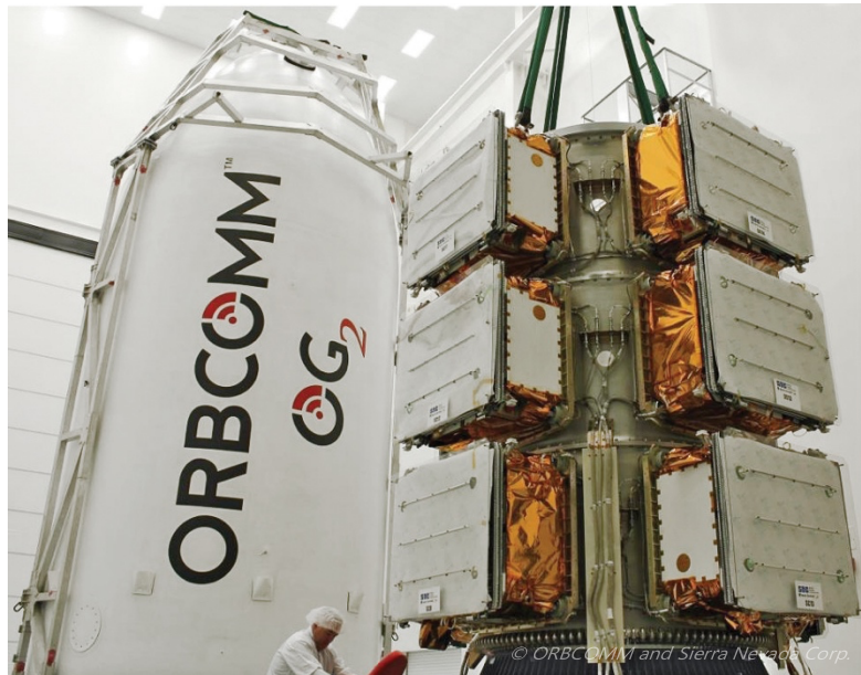
Figure 2. Left, ESPA and auxiliary payloads launching with primary spacecraft Right, ESPA stack for ORBCOMM OG2 spacecraft
