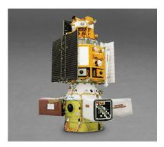
Rideshare Adapters provide space access for satellites by using excess lift capacity to facilitate multiple payloads on a single launch. Moog designed, built, and qualified the Evolved Secondary Payload Adapter (ESPA), and this development spurred Moog's wider product line of adapters for small satellites of all sizes.
