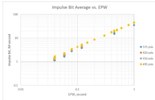
Fig. 11 Impulse Bit Average vs. EPW
