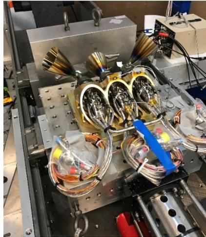
Fig. 5 REM Shock Setup - Moog, Mountain View
