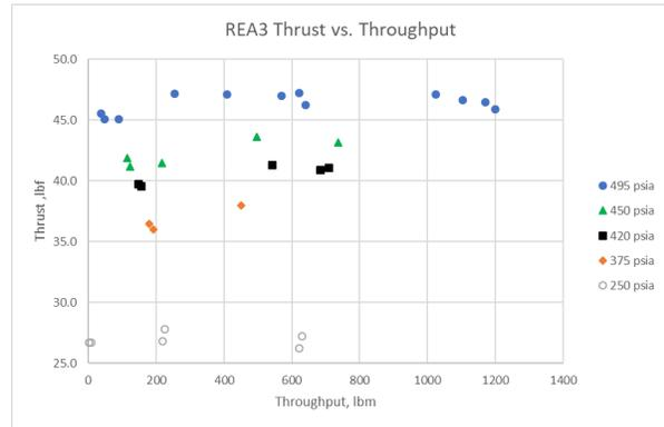
Fig. 10 REA 3 Thrust vs. Throughput
