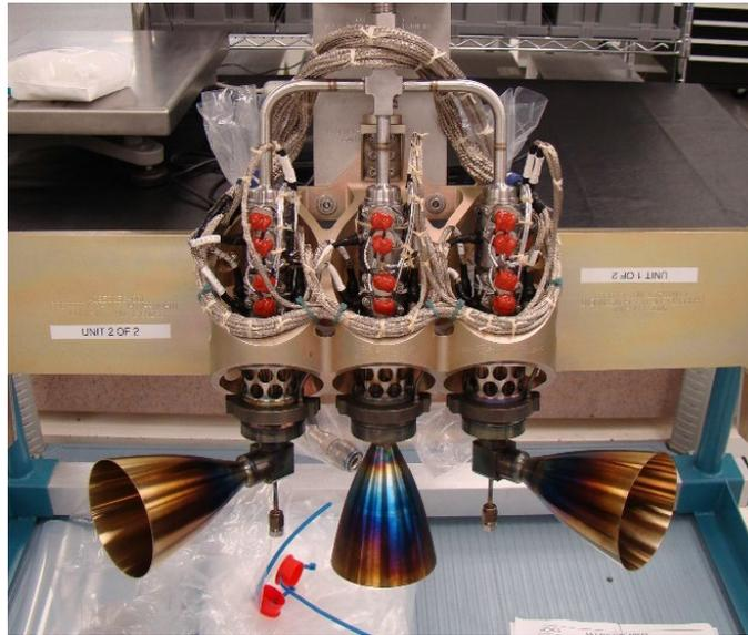
**Fig. 2 Pathfinder Rocket Engine Module**
