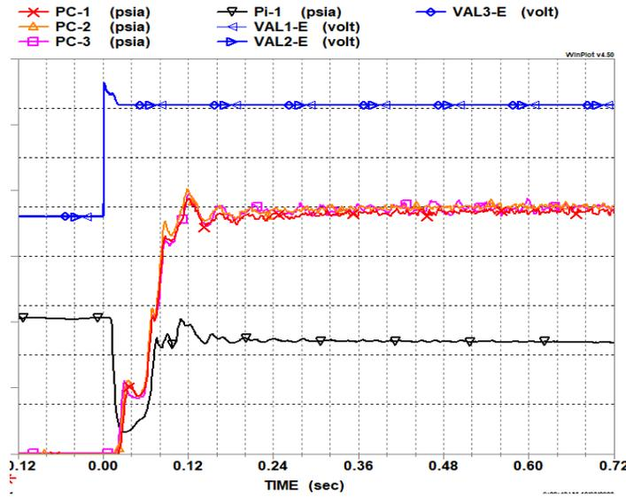
Fig. 15 Multi REA Startup Transient
