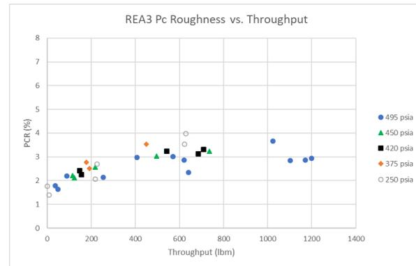
**Fig. 9 REA 3 Pc Roughness vs. Throughput**
