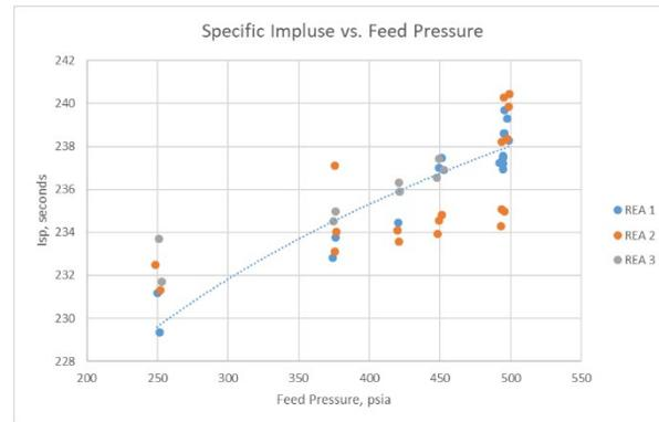
**Fig. 8 Specific Impulse vs. Feed Pressure**
