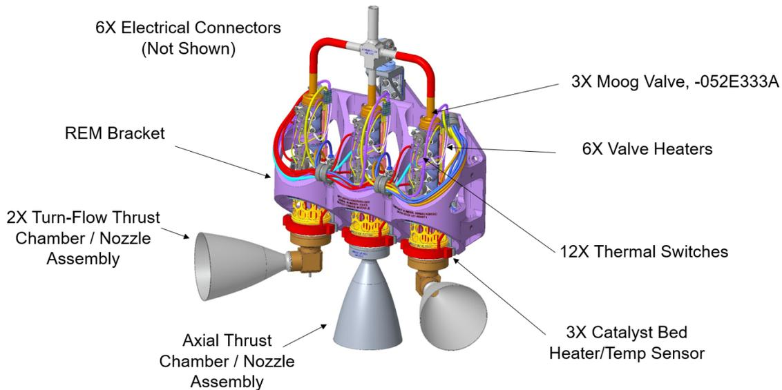
**Fig. 1 Rocket Engine Module Configuration**
