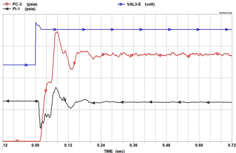
**Fig. 14 Single REA Startup Transient**
