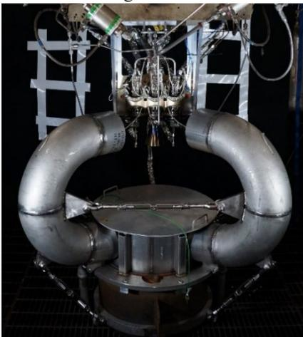
Fig. 6 REM Hot Fire Setup
