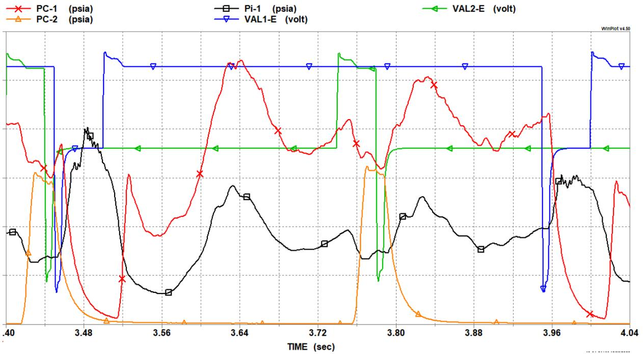
Fig. 18 Multi REA Firing - A2-8792
