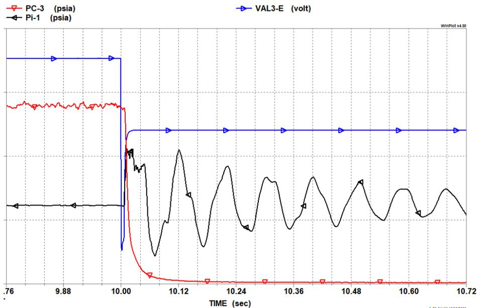
Fig. 16 Single REA Shutdown Transient
