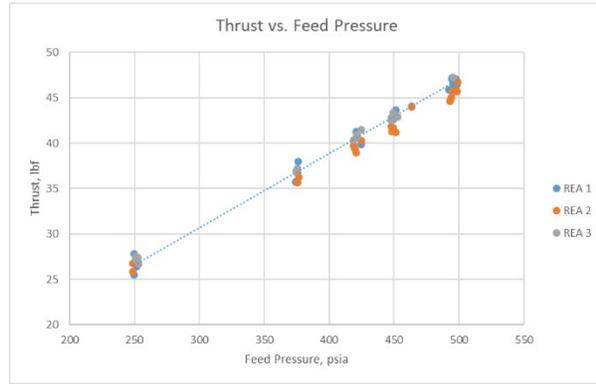
**Fig. 7 Thrust vs. Feed Pressure**
