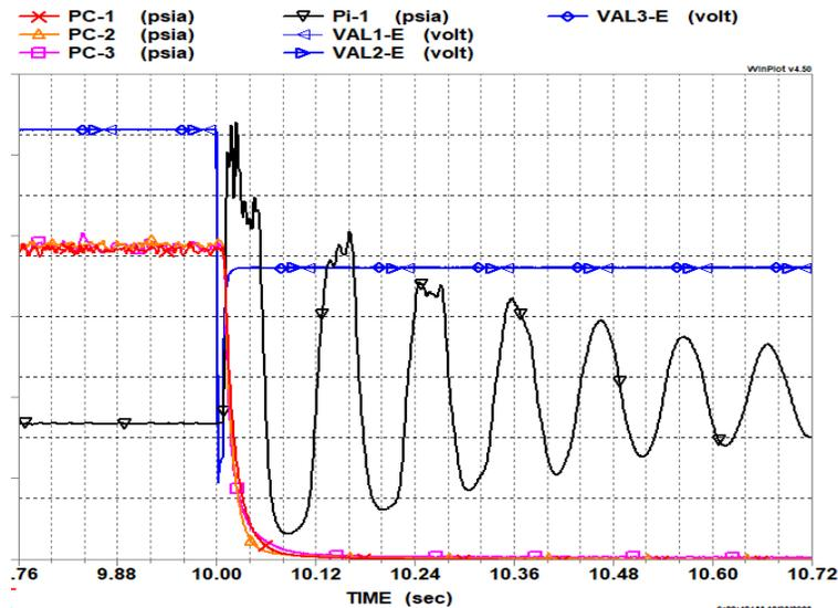
Fig. 17 Multi REA Shut Down Transient
