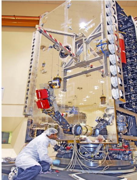
**Figure 1: Mechanical gravity offloader**
