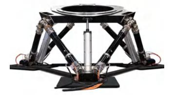
**Driving Simulator with yaw table** 7 DOF motion base with yaw table to simulate city driving.
