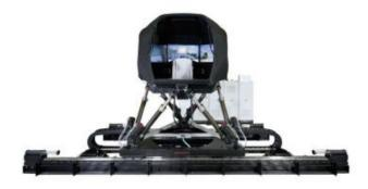
**Fuel Tank Test System** 6 DOF Electric Simulation Table with 2-DOF Tilt Table.
