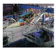
Defence Science and Technology Group (DST): Custom servo actuators and abort manifolds for BAE Hawk Mk 127 Test rig.
