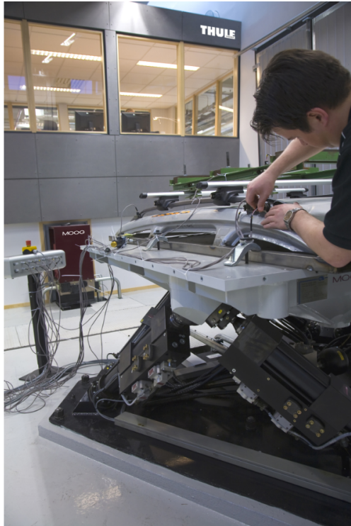
A Thule AB Group Auto Test engineer works with our Moog Hydraulic Simulation Table
